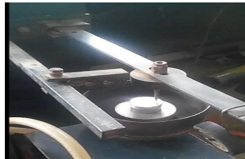
Plate 4: Stationary pin and rotating disc
